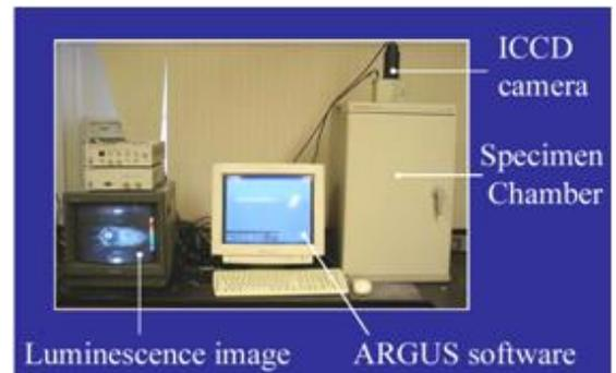
**Fig. 8. Bioluminescence imaging set-up**
