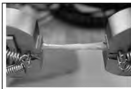
Figure 1 Segment of a human nerve clamped in the tensile testing device
